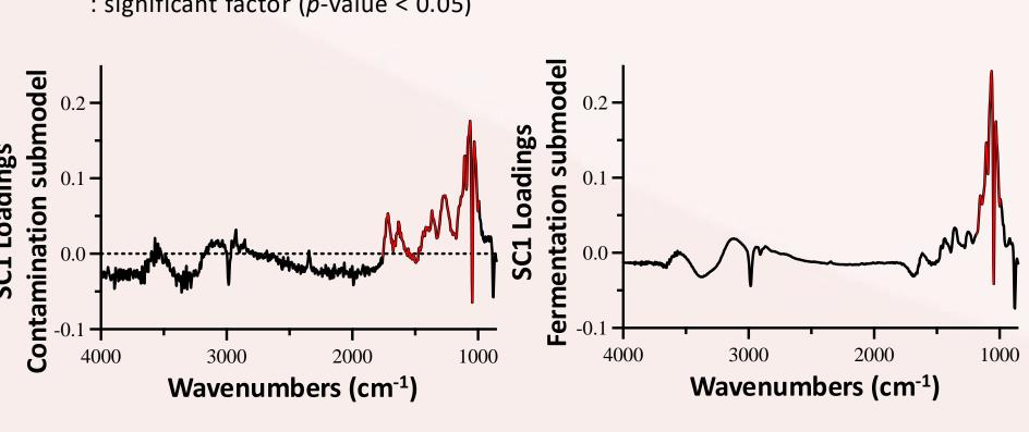
Both process are caused by microorganism, so the spectroscopic fingerprint of both of them overlap
